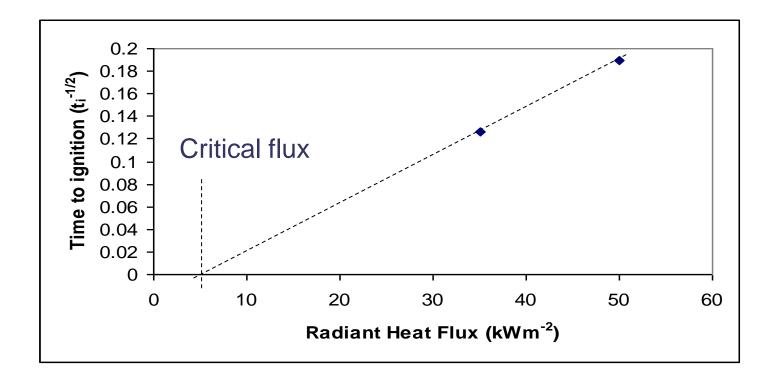
Plotting (1/time to ignition)<sup>1/2</sup> against heat flux shows a value below which ignition does not occur
