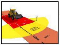
Zone 1 - Always signal the plant operator and receive a positive response before entering Zone 1
