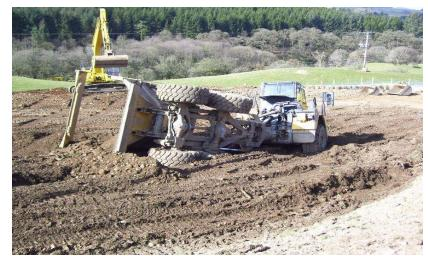
Personal safety should not be compromised, always maintain a safe distance from any vehicles, particularly if they are reversing, and any fixed object and never stand this close when tipping operations are underway, <u>lorries</u> do fall over!
