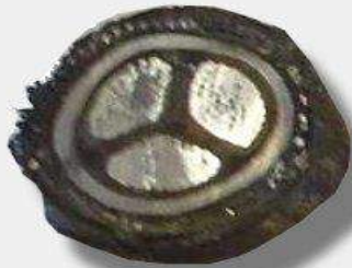
11kV PILC (paper insulated lead covered)
