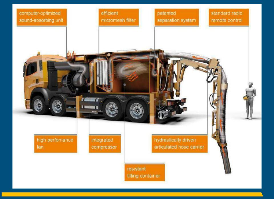
Typically mounted on Rigid chassis 18-32T
