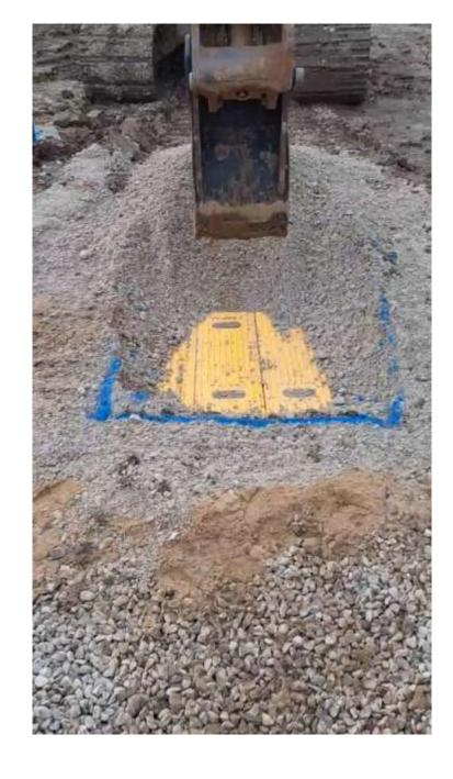
The Video demonstrates the impact resistance of the system with a 16T Excavator exerting maximum force whilst the Strike Matz Boards are fitted in situ.
