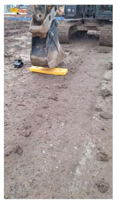
The Video demonstrates the impact resistance of the System with a 16T excavator exerting maximum force on a concrete surface to test the braking force of the System.
