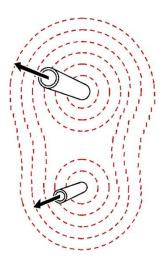
Distorted signals can cause inaccuracies when marking out, and with depth estimations
