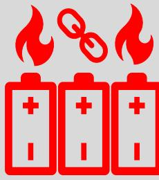
The chain reaction spreads to adjacent battery cells.
