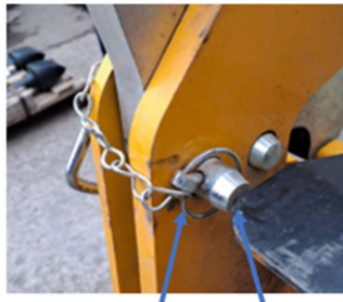
JCB retaining/linch pin and main lock pin securely in place. Additional JCB securing chain should also be attached (as above)
