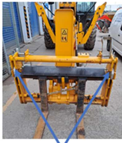
JCB Telehandler with retaining/ linch pin and main lock pin in place
