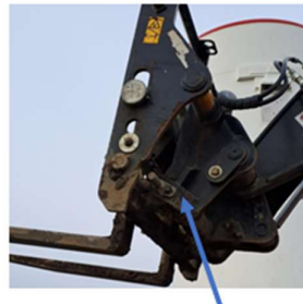
Manitou Telehandler with retaining/ linch pin and main lock pin in place
